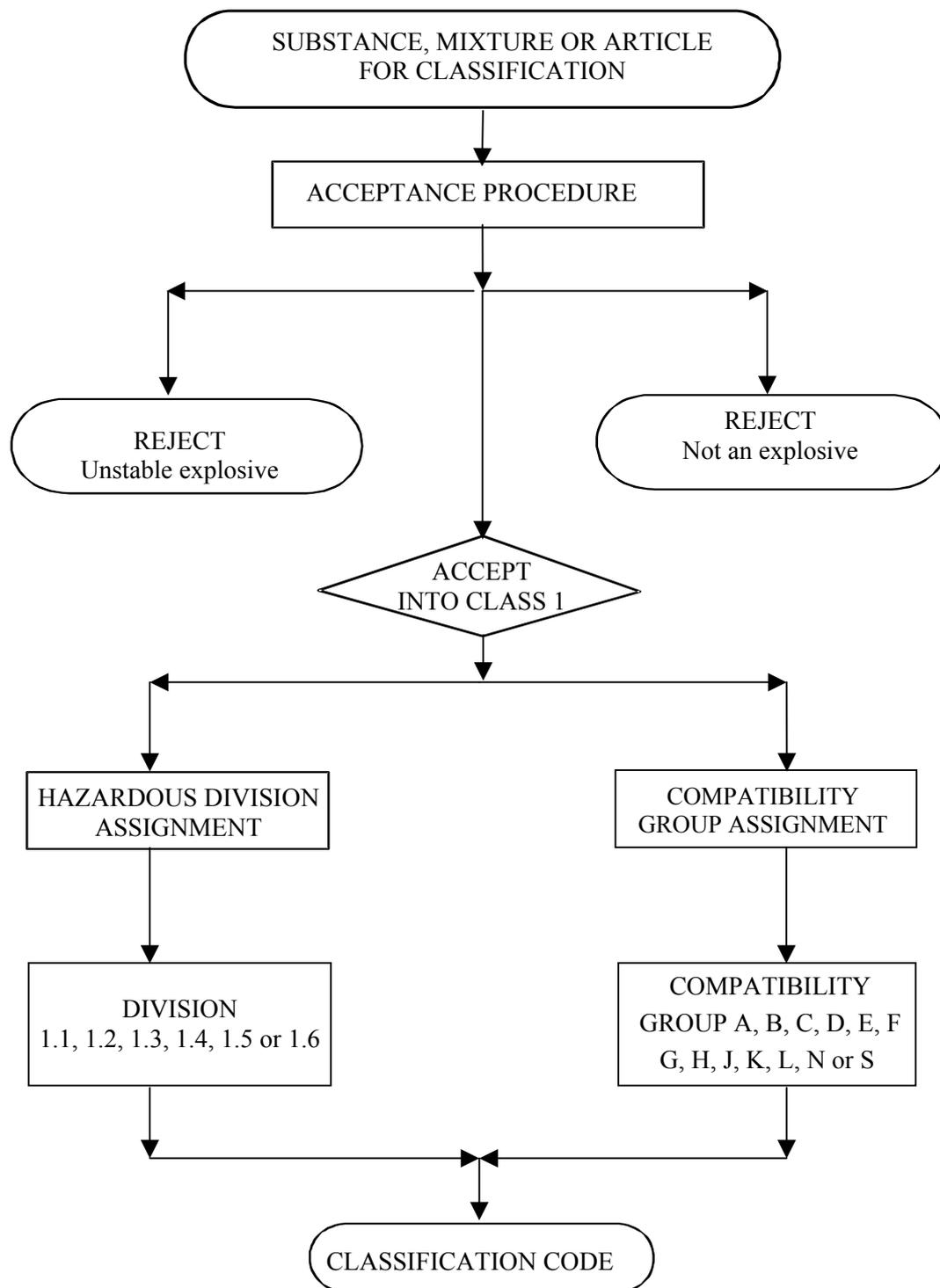
**Figure 2.1.2: Procedure for provisional acceptance of a substance, mixture or article in the class of explosives (Class 1)**
